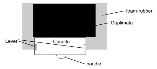
The handle can be pulled to its outer position as soon as the machine has completed a duplicate. Once the handle is pushed to its inner position, the machine will start dealing the next duplicate. This gives you two possibilities:
