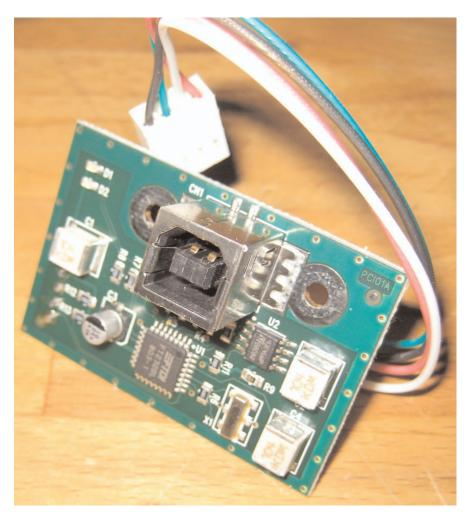
The USB kit is a small PCB that sits on the inside of the machine's back panel, see the illustration to the right at the bottom of the page.
