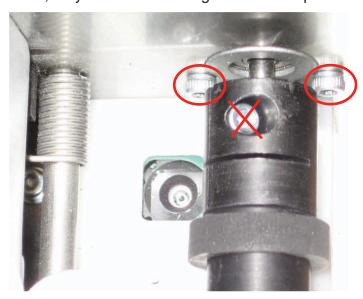
There are holes in the front panel though which you can insert a (long) allen key, see the illustrations below.
