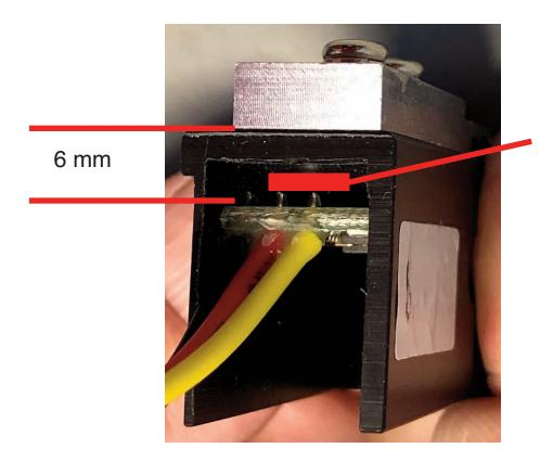
The reader must be mounted with a 1 mm thick double adhesive tape (or it will be out of focus).
