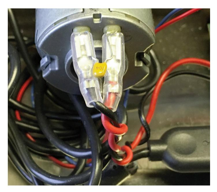
The two (red and black respectively) power cables should be twinned as shown above and there should also be a resistance between the two poles. Be careful to keep the resistance flat over the contacts as shown above. The motor will go in spin if you connect the resistance with earth (i.e. if you let it come in contact with the motor).
