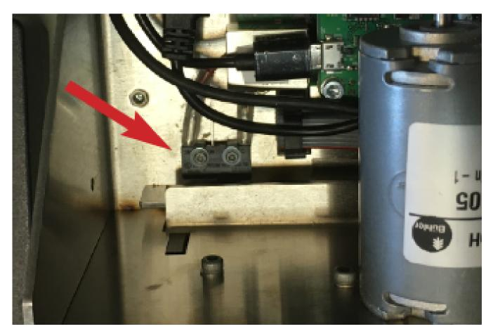
Lock the screws and test that the switch is correctly positioned before tightening the two screws.
