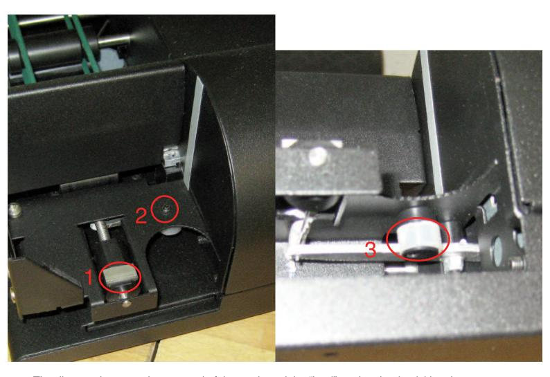
The distance between the rear end of the cards and the "heel" on the shuttle picking the cards from the hopper needs to be correctly adjusted.
