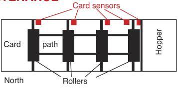
The counters are numbered in the same way as the cards move from the hopper to the left, i.e. in the cards' direction.
