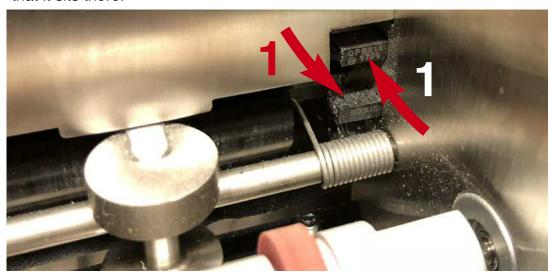
Make sure that you clean all five sensors with compressed air while you are at it. You can use a small soft brush (e.g. a childs tooth brush) if you do not have access to compressed air.
